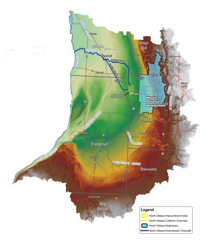
An 8.5-mile-long collection channel intercepts the westward flow of existing ditch laterals and diverts the flow to a 1.5-mile-long inlet channel, diked on both sides, that conveys water to the impoundment.
